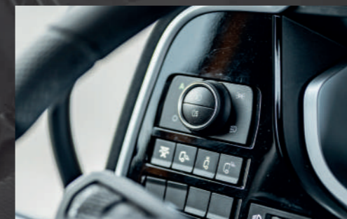
External illumination control
